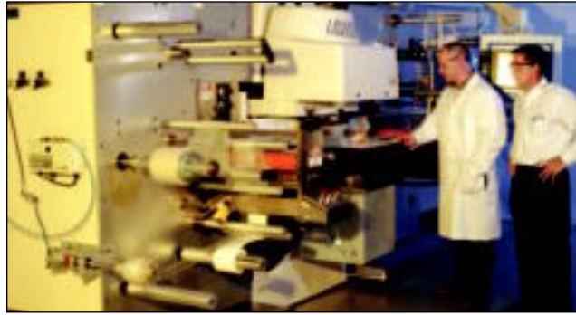
Figure 1. A roll-to-roll laser digital converting system. The laser processing module (LPM) is located between the material unwind and rewind modules.
