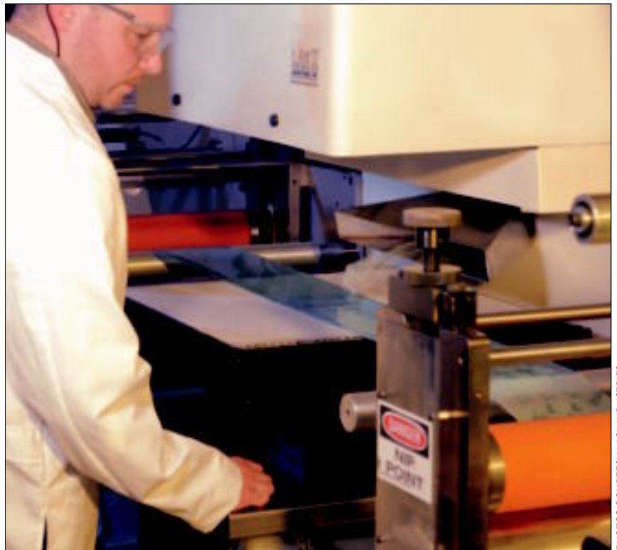
A process engineer monitors the production run of microassay subcomponents on a LaserSharp digital converting system by LasX Technologies.
