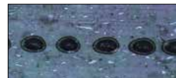
Gaps due to poor laser beam control.
