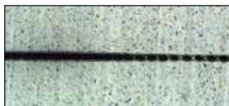
Inconsistent scoring at varying production speeds.
